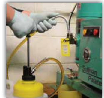
Compressor being filled with a Spectrum Container using the hand pump
