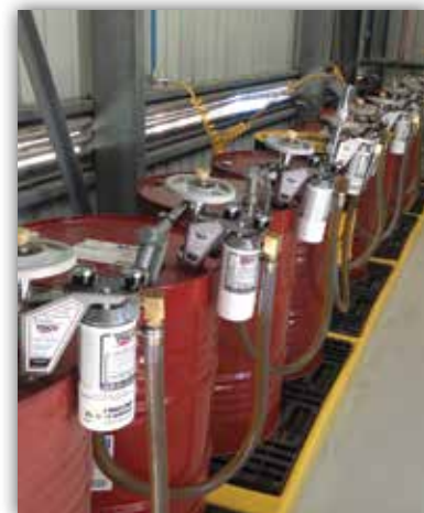
Electric Pump Motor installed on Drum Pump Filtration System
