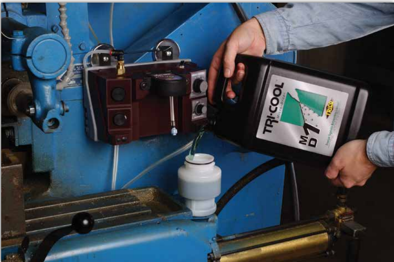
Micro-dispenser being filled with Tri-Cool MD-1 lubricant
